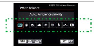
colours, the camera should be **white balanced**. This can be done in the camera menu by changing the Kelvin temperature of the light source, or, for more precise adjustments, with the camera control software on the computer. With the Canon EOS Utilities software, for example, the white balance can be adjusted with the **eyedropper tool**. Just use a white object as a reference, and with one click, the white balancing is done.
