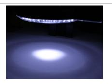
By adjusting the ring light to the optimal working distance, you get an evenly illuminated visual field in the area captured by the camera.
